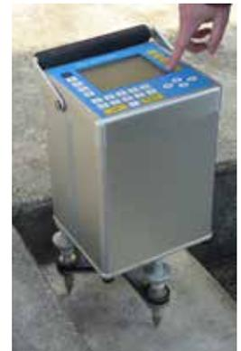
Fig 6. Gravity meter
