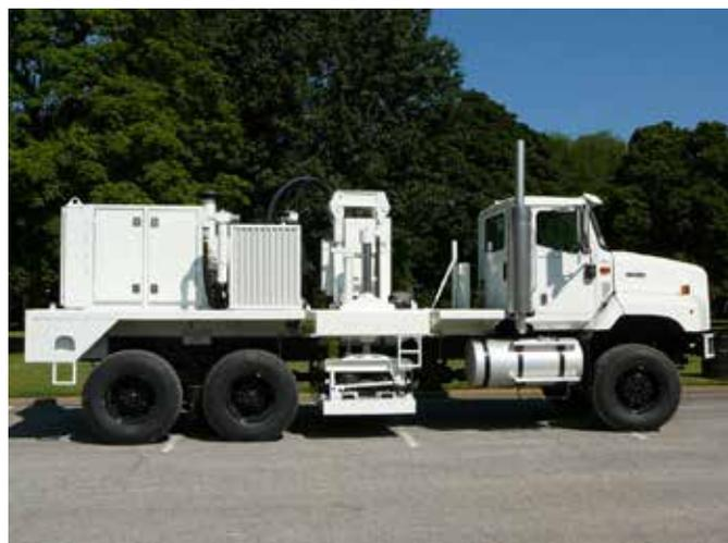
Fig 2. Three Vibroseis trucks are used for a seismic survey
